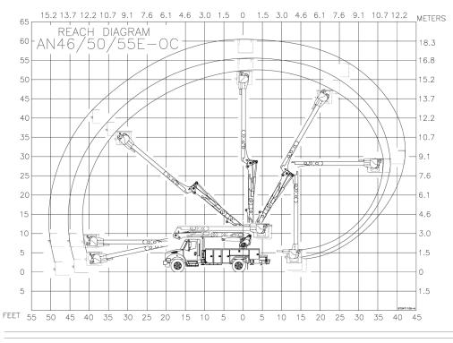
OPTIONAL JIB PLACEMENT BETWEEN ONE-MAN PLATFORM AND BOOM TIP
